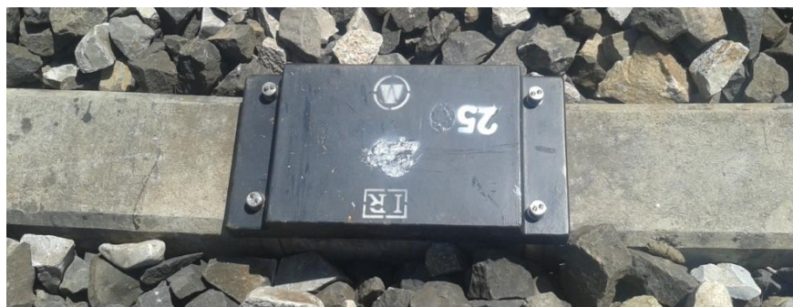
Figure 7: RFID Tag fixed on sleeper
